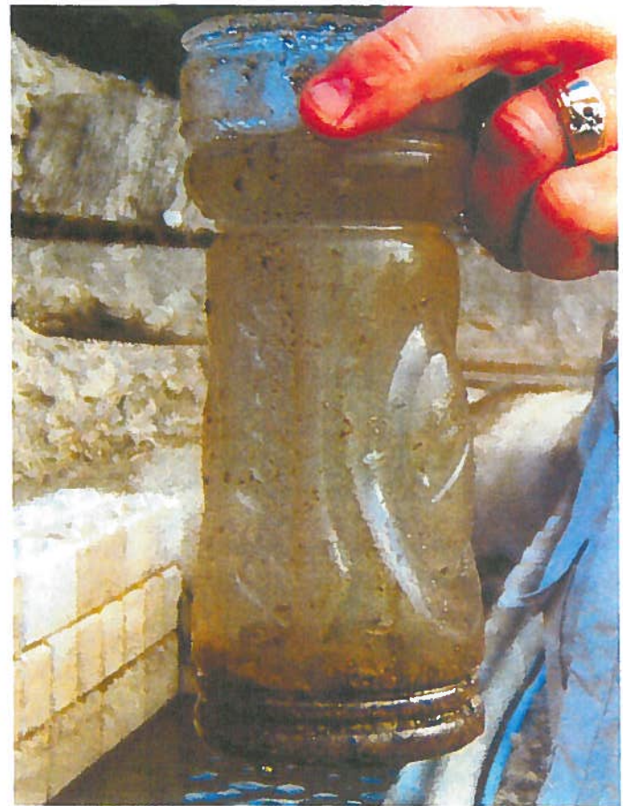
Within the floc sand pond, floc-sand precipitates almost immediately out of the treated water as 1-2 cm diameter pellets.
