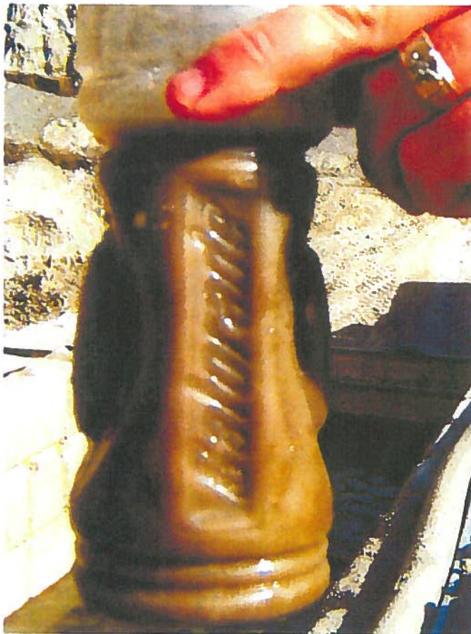
Within the floc sand pond, floc-sand precipitates almost immediately out of the treated water as 1-2 cm diameter pellets.
