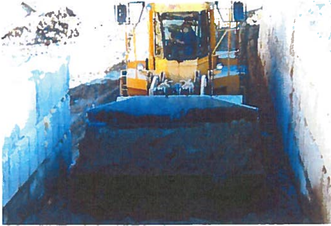
The early stability of the floc-sand is a big factor in the system's success. Each day's accumulation can be dug out of the floc-sand pond the next morning.
