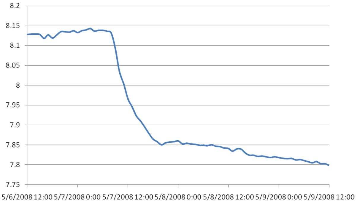
**Figure 2 Coquitlam River stage elevation decrease during rampdown May 7, 2008.**
