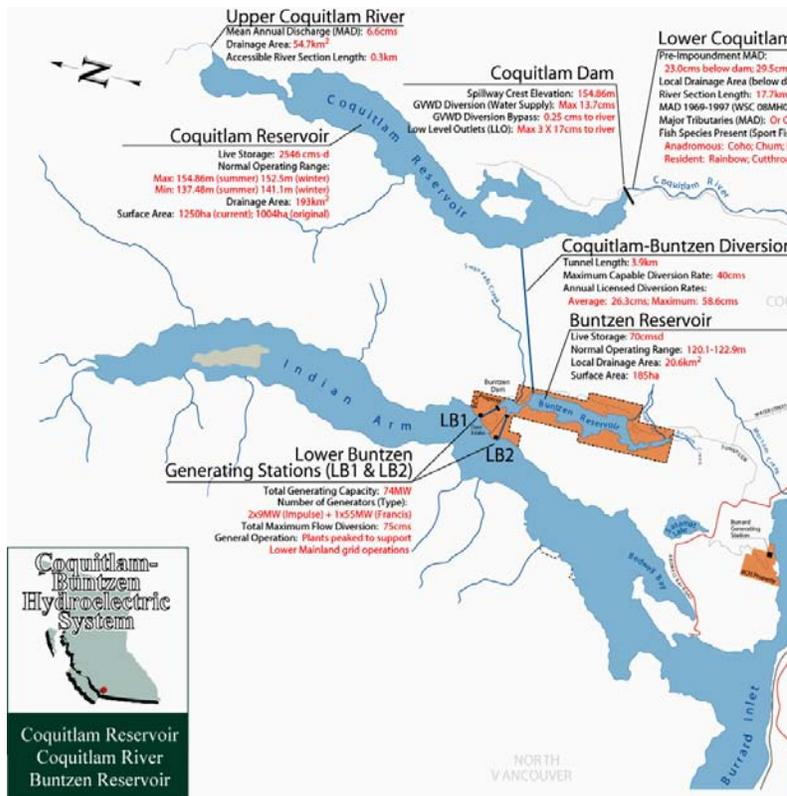
**Figure 1 Coquitlam-Buntzen Reservoir, Diversion and Generating System**
